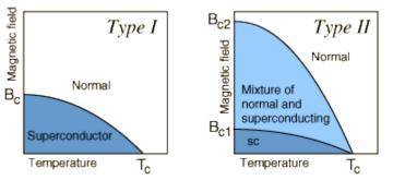
It is the nature of superconductors to exclude magnetic fields (Meissner effect) so long as the applied field does not exceed their critical magnetic field. This critical magnetic field is tabulated for 0K and decreases from that magnitude with increasing temperature, reaching zero at the critical temperature for superconductivity. The critical magnetic field at any temperature below the critical temperature is given by the relationship
